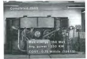
Figure 1.9 The second Harvard Cyclotron with a proton energy of 160 MeV. The first cyclotron had been dismantled and moved to assist in the Manhattan project.
